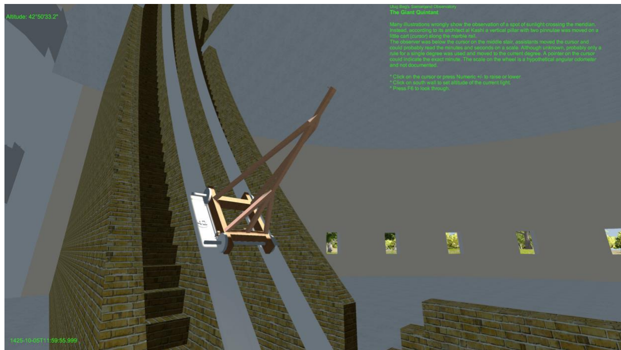
Figure 9. The observing cart in the virtual reconstruction of the central meridian instrument of Ulugh Beg's Samarkand observatory [Zotti and Mozaffari 2020] can be moved by the visitor along the curved rails cut into the marble surface of the 40 m arc. Looking through the sights onto the sky provided by Stellarium allows the recreation of the historical observations from its heydays (around 1430 AD). In this scene, a patch of sunlight crosses the meridian arc at local noon. The cart, for which proof has been found in a manuscript, has been positioned to measure the transit altitude. The observer would have been placed on the central staircase, while the cart would have been operated by two assistants in the side staircases and probably secured by bolts. The model also allowed developing the authors' conviction that this instrument was not a full quadrant, given that the cart would not be usable in the vertical uppermost parts of the instrument elsewhere hypothesized as complete quadrant. The image has been brightened up for reproduction.
