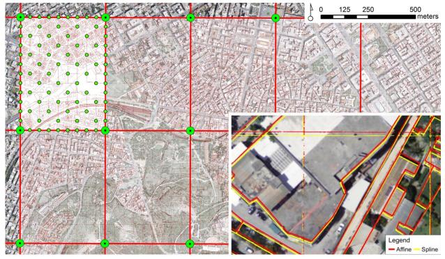
Figure 4. Part of the georeferenced raster collection of the 1972-76 cadastral distribution (Ministry of Public Works) for the center of Athens. Distribution of points used in the georeferencing process is indicated at the top left map sheet, while the results of spline and affine transformations are compared in relation to satellite imagery (detail at bottom right).
