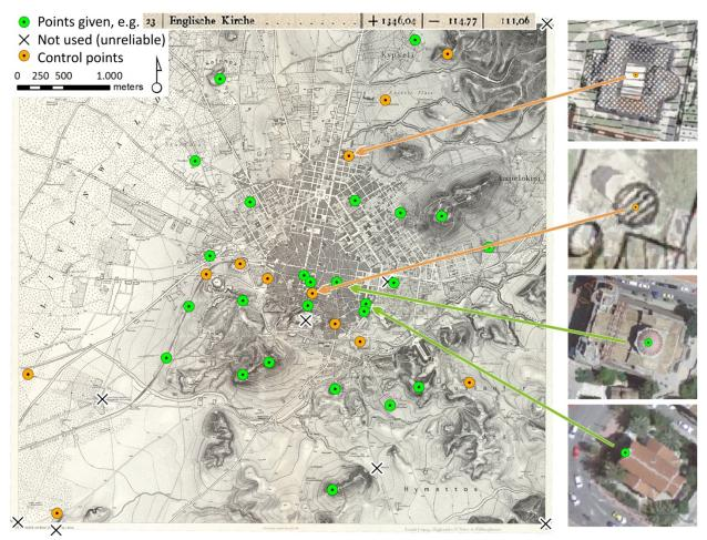
Figure 6. Georeferenced map sheet I from Karten von Attika [Curtius and Kaupert 1881]. Deviation of points used in the transformation procedure and control points are displayed on the satellite imagery (at right).
