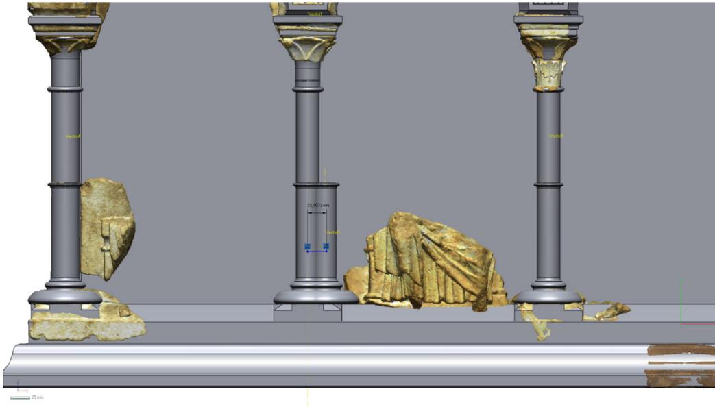
Figure 10. Modified distance between the columns in the new reconstruction. The size and position of a carved element changes the distance between the columns, previously only identified by the size of the reconstructed trefoil arch.
