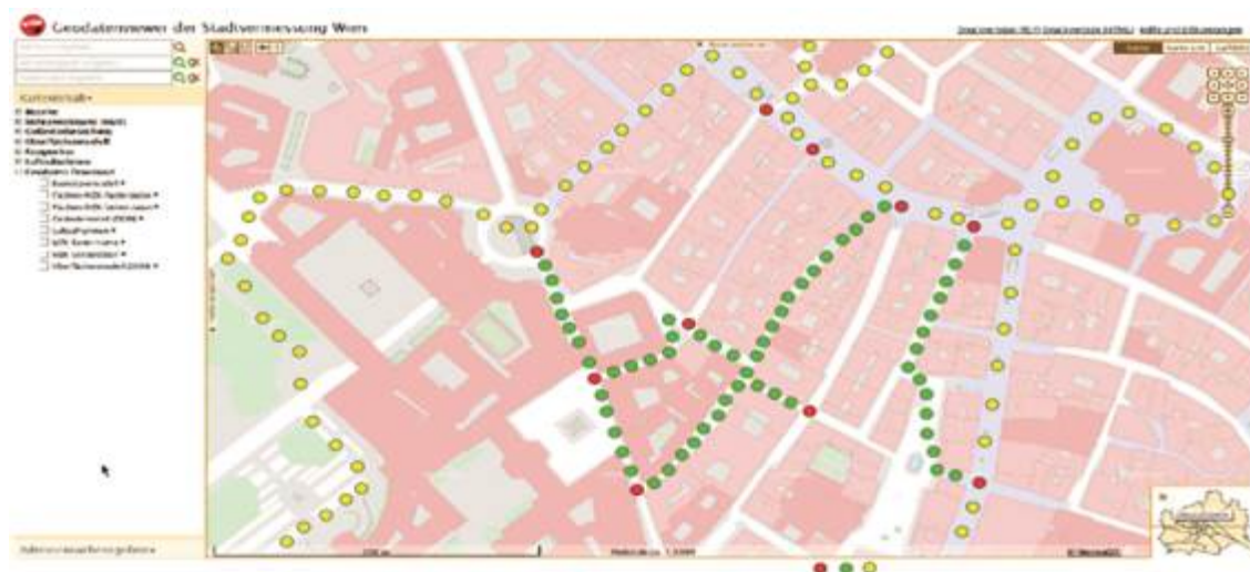
Figure 13. Schematic of new Workflow. Red points: registered cross-way scans. Green points: connecting scans between cross-ways (registered in RiSOLVE).
