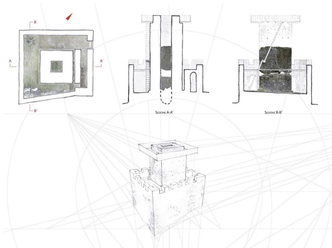
Figure 16. Draft reconstruction of the northern tower.
