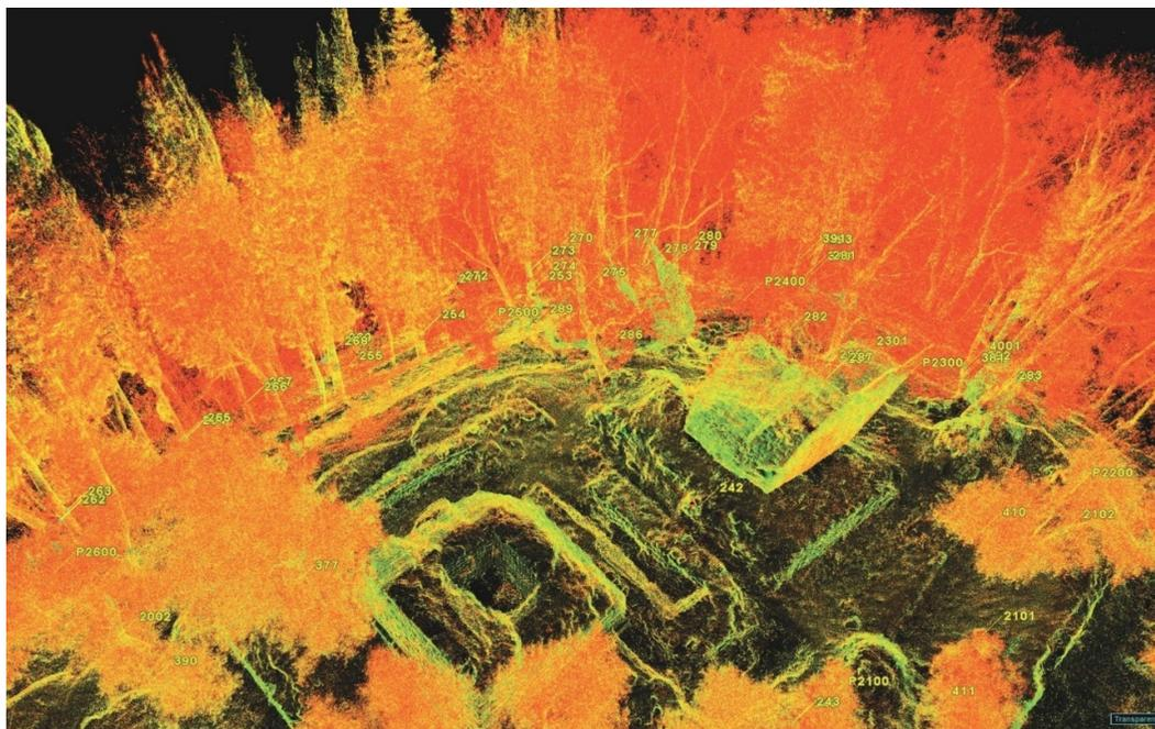
Figure 7. The general aligned point cloud from the 3D laser scanner survey, view of the northern tower.
