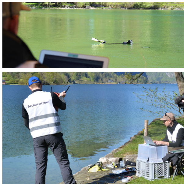
Figure 7. The base camp, placed to the north of the site, provides a workplace for the operator ("pilot"), who remotely controls the UUV via a laptop. Lower right: Equipment containers conveniently double as mobile control desk. "Copilot 1" stands close to the base to manage the cable and communicate via gestures with the UUV's supporter/diver. Similar to UAV-based documentation, when no live information about the UUV's current position is available, a second copilot is placed to the side of the surveyed area and provides an estimation of distance.
