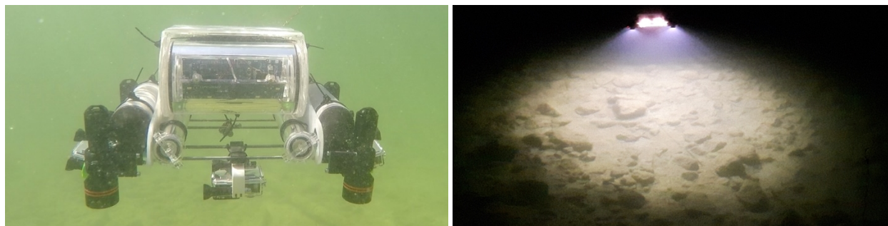
Figure 5. The images show “Eckbert-II” submerged in Lake Mondsee. Left: A flexible camera- and lighting setup can accommodate different recording needs and environmental conditions. To document the pile dwellings, three GoPro Hero 4 BE were attached to the UUV. Subsequently, weights and buoyancy bodies were combined to balance the UUV. Right: Recording can be done in complete darkness, thanks to the diving torch setup used. Under these extreme conditions, 3d models can still be produced successfully.
