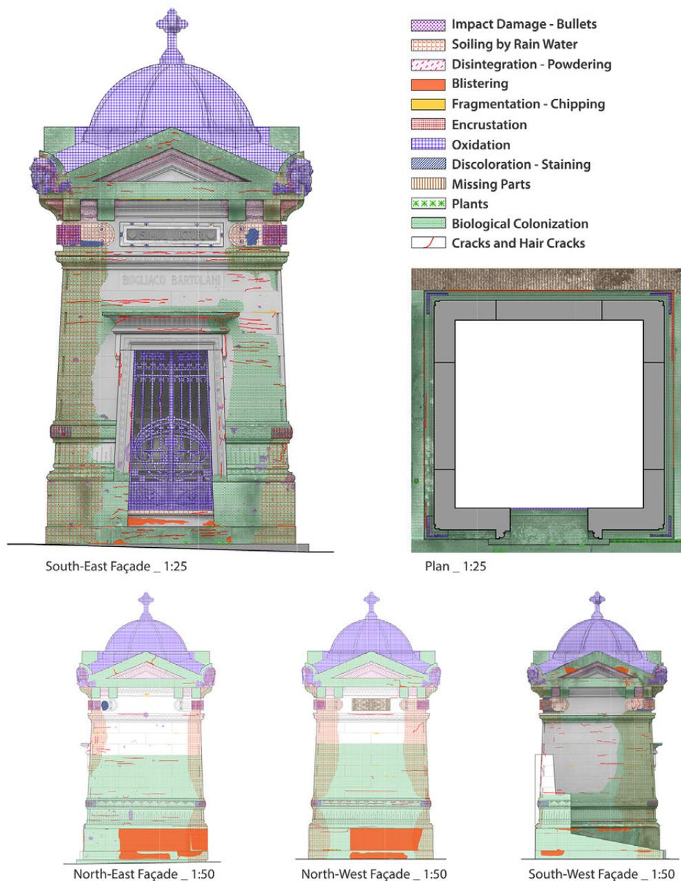
Figure 10. Deterioration mapping of the facades of the Bartolani chapel.
