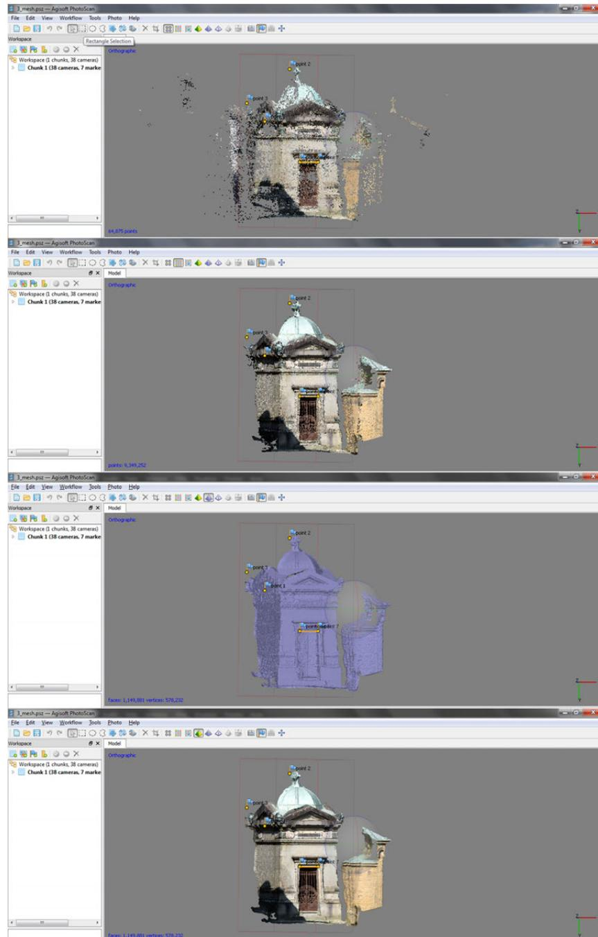
Figure 7. Phases of the photogrammetric survey of the Bagliaco Bartolani Chapel.
