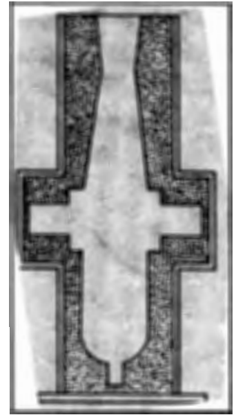
Figure 11: Cross section of a gun flask.
