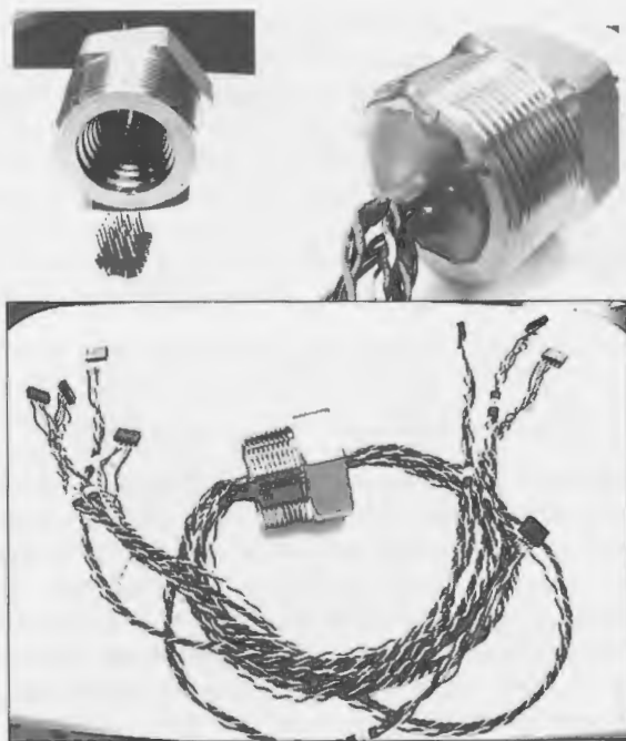
Figure 7. Test Cylinder Feedthrough: (clockwise from upper left) tapered cone drilling of nut and group of 4 pin connectors to be sealed inside the nut; wires soldered to pin connectors and encased in J-B Weld inside the hollow plug; full feedthrough containing 4 sets of wires.
