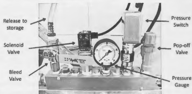
Figure 5. Manifold with components noted.
