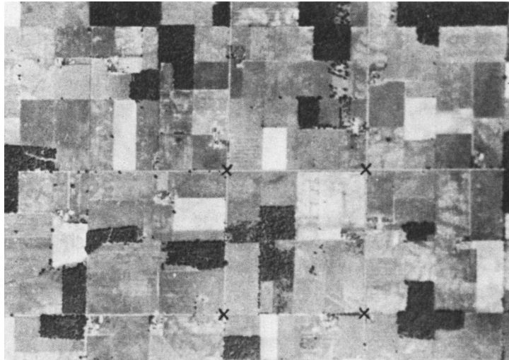
AERIAL PHOTOGRAPH OF AN AREA IN NORTHWESTERN OHIO SUBDIVIDED IN THE MANNER OF THE UNITED STATES LAND SURVEY SYSTEM. The black crosses indicate a quarter section ( \frac{1}{2} \times \frac{1}{2} mile).
