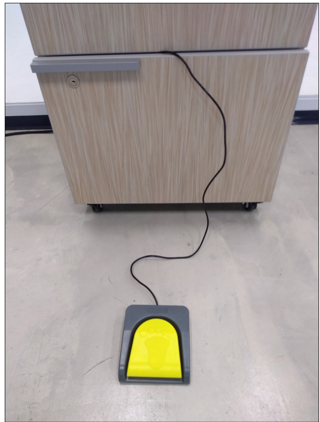
FIGURE 9. The kiosk's USB foot pedal partially extended from the kiosk. It can extend approximately six feet from the kiosk but can be extended farther through the use of USB extender cables.
