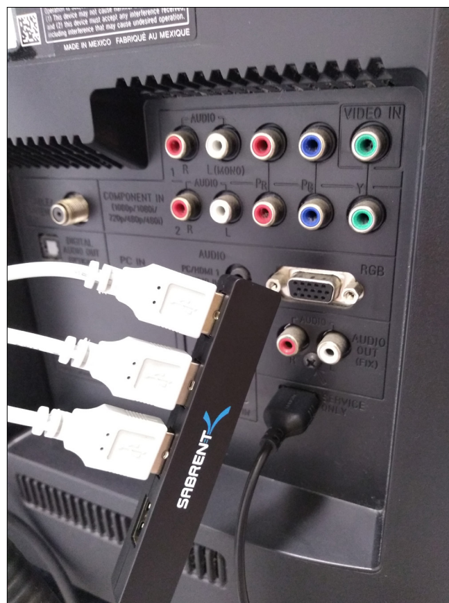
FIGURE 3. The use of an unpowered USB hub was necessary to connect all three USB lights to the single USB port on the back of the television. The lights are powered down when power to the kiosk is lost.
