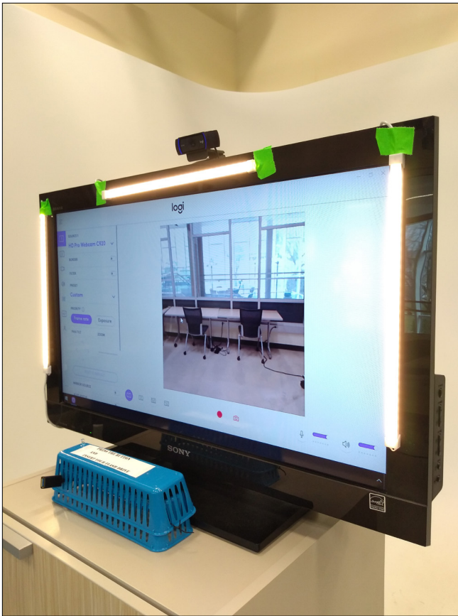
FIGURE 4. The television used with the kiosk, showing the attached LED lights and its orientation at the top of the kiosk.
