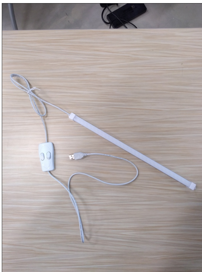
FIGURE 2. An example of one of the three USB lights used with the kiosk, selected for this project based on the binary switch. The switch remains in the “on” position at all times, allowing the lights to be powered down when power to the kiosk is lost.
