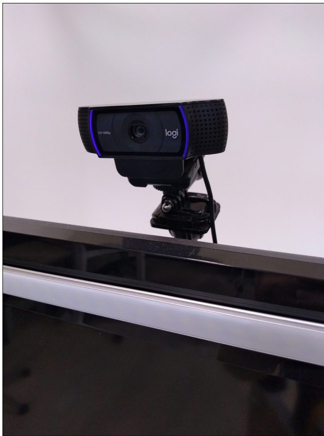
FIGURE 8. The web camera used for the kiosk. While it is currently positioned directly above the television, its flexible mount allows for its position to be moved in a variety of other orientations
