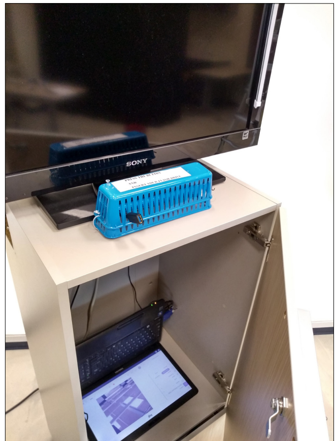
FIGURE 7. A look at the laptop currently powering the kiosk. As can be seen, there is space for placement of a regular desktop computer in later iterations of the design.
