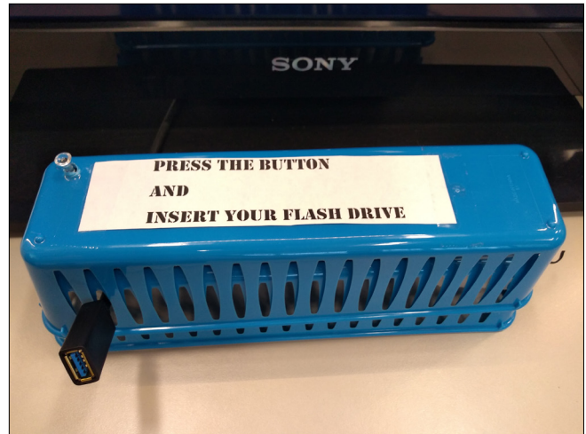
FIGURE 6. The remote control enclosure as it appears when ready for use, showing both directions and easy access for users to plug in their flash drives.
