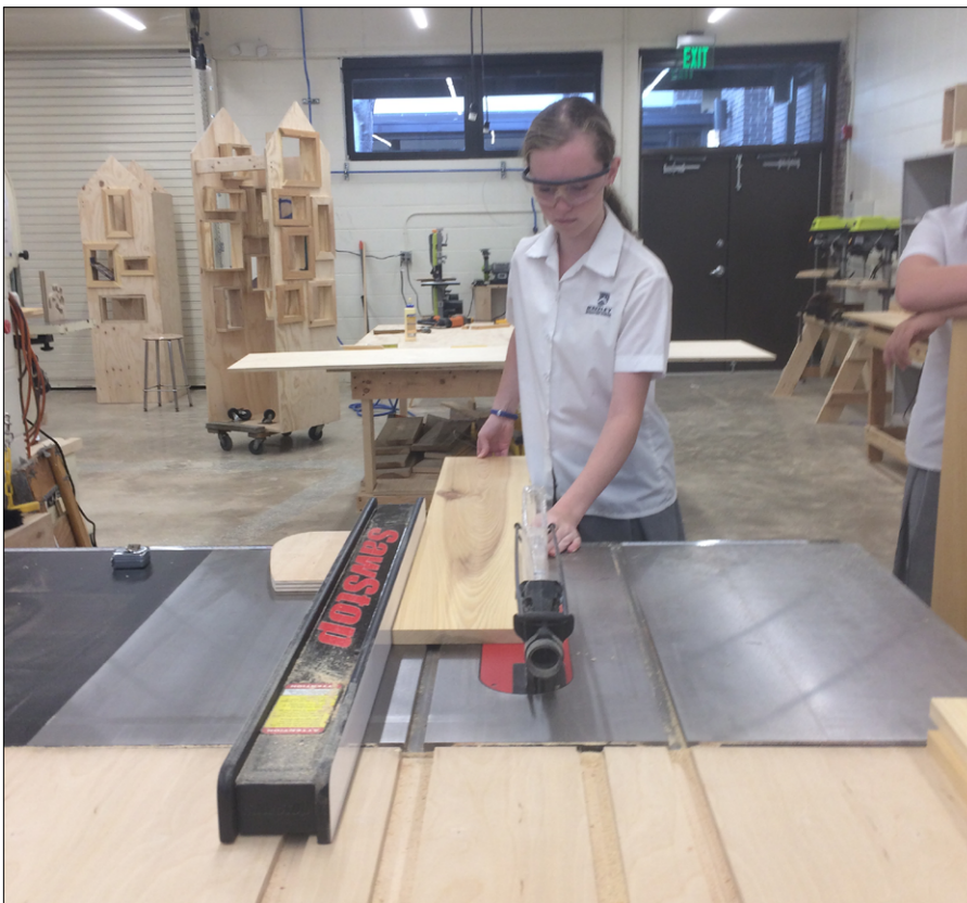
FIGURE 11. Eighth-grade student using the table saw to cut milled lumber to exact size for a chair project.
