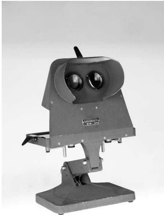
Figure 2. A Davidsen-Wottring caecanometer. LeRoy Wottring of the Wottring Instrument Company patented this device in 1951. 13 Wottring also invented the Rotoscope 16 and Troposcope 17 , instruments used for diagnosing and treating binocular vision problems.
