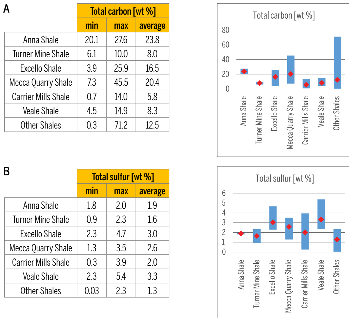
Figure 3. Table data and graphs showing the total carbon and total sulfur content (ranges and average values, uncertainty \pm 0.02 for C and \pm 0.04 for S) in the shales studied.
