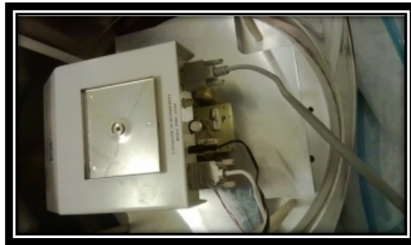
Figure 6- MSB device positioned in the mu-metal shielding
