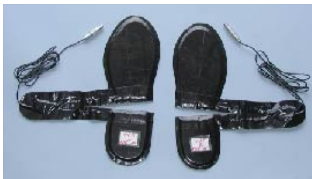
Figure 4. Insoles containing foot switches for stride analysis.
