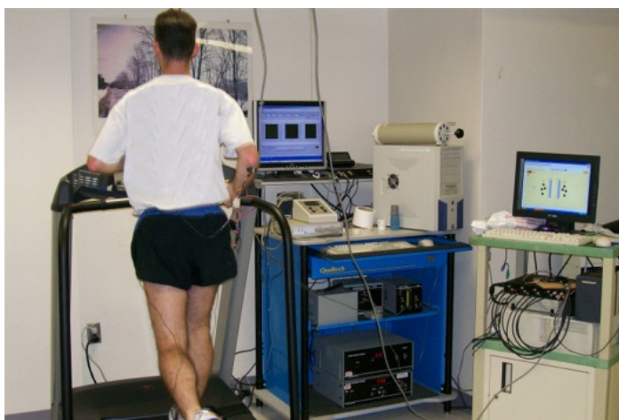
Figure 5. Experimental set-up. While subject ran on the treadmill, metabolic data ( \dot{V}O_{2\text{max}} , economy) were collected by the left computer and entrainment data were collected by the right computer.
