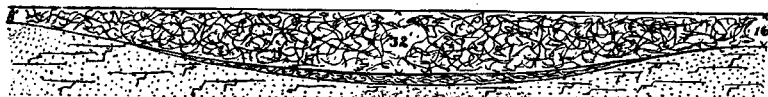
Fig. 5. Ideal section of a peat bog filling a rolling basin or hollow in the sandstone.
