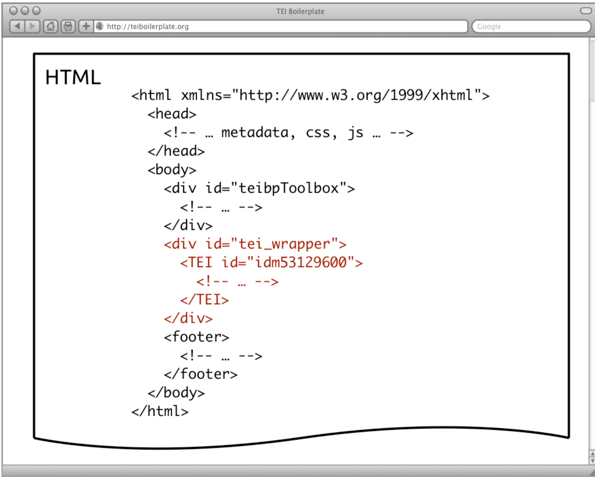
Figure. Through a simple XSLT transformation, the original TEI document is embedded within an HTML5 document. The resulting HTML/TEI document can then be styled with CSS and manipulated with JavaScript as one would an more familiar HTML document.
