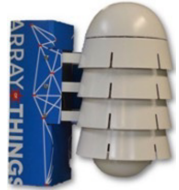
Figure 1: An Array of Things node. In the blue enclosure: edge computers, upward-facing camera, and light sensors; in the white enclosure: a cellular modem, street-facing camera, and environmental and air quality sensors. (Image © University of Chicago, used with permission)
