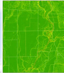
Above is a LiDAR map, (Light Detection and Ranging), that shows where there are differences in elevation.
