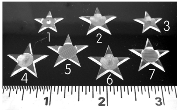
Figure 5: Test of the You Are Here symbols used on Talking Kiosks. Symbol 4 was selected by most people as the clearest indicator of a map reader's current position.
