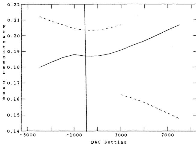
Figure 1. Measured fractional tune vs. quadrupole strength (arbitrary units). The solid line is the "horizontal" and dash-dot line the "vertical" fractional tune.
