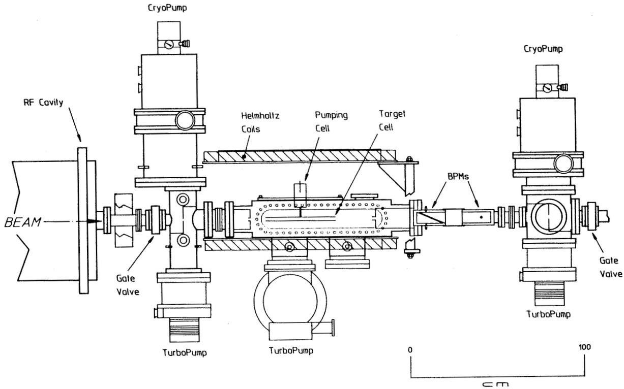
Figure 1. The polarized  $^3\text{He}$  target setup for CE-25 setup in the Cooler A-section.
