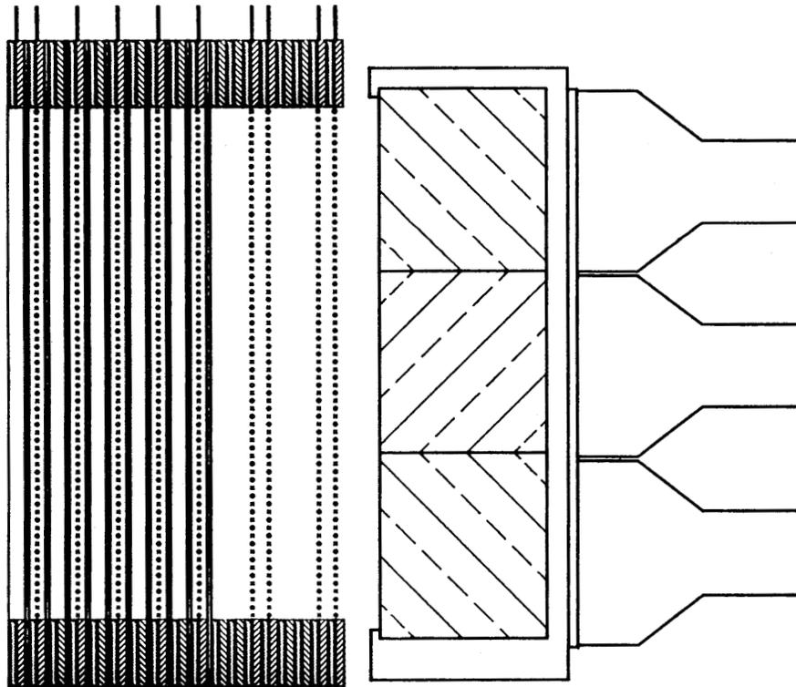
*Figure 1.* Top view of the E358 neutron detector showing the stacking arrangement of the 18 MWPC's followed by the 3 $\times$ 2 array of sodium iodide.
