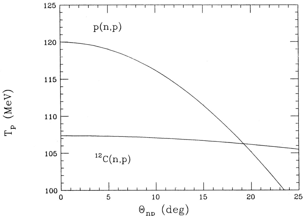
Figure 2. Proton kinetic energy vs. np relative angle for the primary np free scattering reaction and the  $n + {}^{12}\text{C}$  competing background reaction at  $T_n = 120$  MeV. The threshold is due to the difference in  $Q$  values for these processes.
