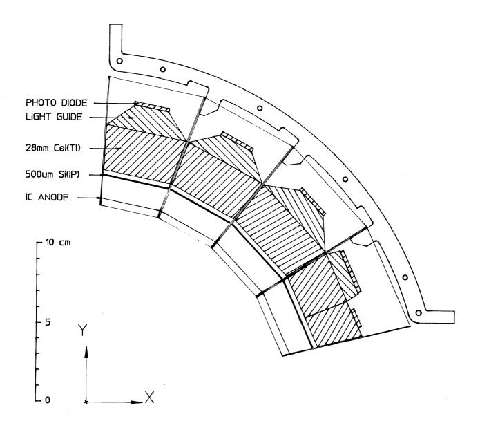
Figure 2. Telescope configuration for forward hemisphere array. Each unit is part of an 18-member ring; forward-most element is segmented into two halves.
