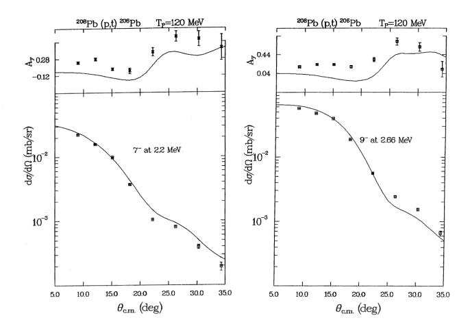
Figure 1. Experimental cross sections (full dots) and analyzing powers (open dots). Zerorange DWBA calculations (full line).
