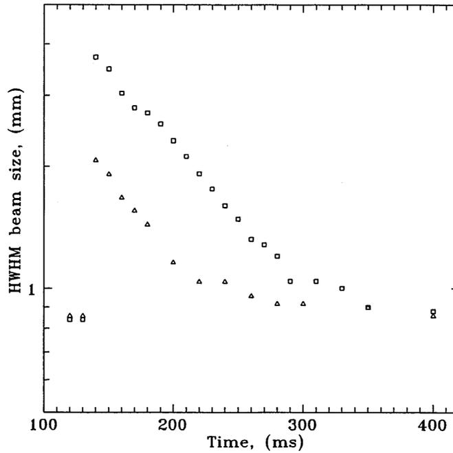
Figure 4. Transverse proton beam profile (HWHM) as a function of time for two different kick strengths. The transverse kick occurred at 140 ms.
