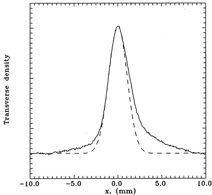
Figure 1. Transverse beam profile (solid) and Gaussian fit (dashed). Average (peak) beam current: 460 (2,000)  $\mu\text{A}$ ; rms size from the fit: 1.05 mm.
