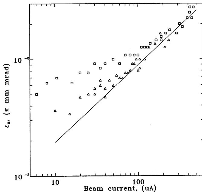
Figure 2. Normalized rms emittance as a function of the average bunched proton beam current before ( $\square$ ) and after ( $\triangle$ ) the alignment of electron and proton beams. Solid line is  $I^{2/3}$ .
