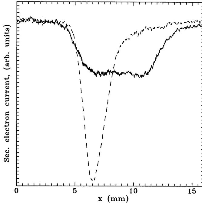
Figure 3. Secondary electron current produced by the filament traversing the proton beam immediately before (dashed) and immediately after (solid) the transverse kick.
