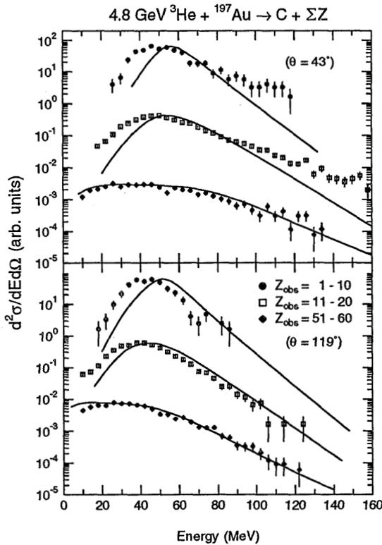
Figure 2. Laboratory energy spectra of carbon fragments from the 4.8 GeV  ${}^3\text{He} + {}^{197}\text{Au}$  reaction, gated on total observed charge. Points are for  $Z_{obs} = 1-10$  (top);  $Z_{obs} = 11-20$  (middle) and  $Z_{obs} = 41-50$  (bottom). Lines are predictions of the INC/EES model, normalized so that the maximum probabilities are equal.
