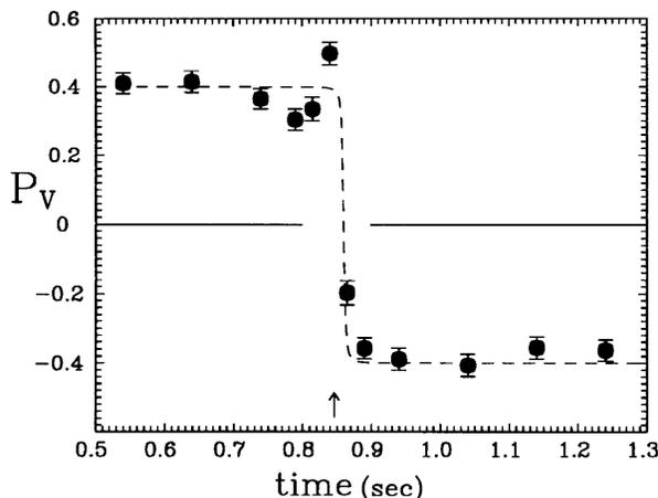
Figure 3. The measured vertical polarization at 380 MeV is plotted against the time of the vertical beam kick. The kicker magnet strength was 0.45 T·mm. The betatron tunes were fixed at  $\nu_y = 4.80$  and  $\nu_x = 3.77$ . The arrow shows the predicted position of the  $G\gamma = 7 - \nu_y$  resonance. The dashed lines are a hand-drawn curve to guide the eye.
