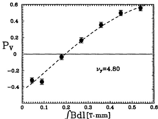
Figure 2. The measured vertical polarization at 380 MeV is plotted against the strength of the vertical kicker magnet in T·mm. The beam was kicked at 0.84 s, while the betatron tunes were  $\nu_y = 4.80$  and  $\nu_x = 3.77$ ; the dashed curve is a fit to Eq. 3 using  $\epsilon = 6.2 \cdot 10^{-5} + 2.4 \cdot 10^{-4} \int B \cdot dl$  [T·mm] and  $\alpha = 2.7 \cdot 10^{-8}$ .
