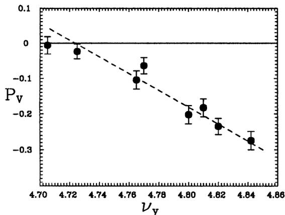
Figure 1. The measured vertical polarization at 380 MeV is plotted against the vertical betatron tune  $\nu_y$ . The horizontal betatron tune  $\nu_x$  was about 3.785. The dashed line is a linear fit suggesting emittance growth during acceleration.
