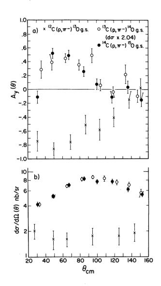
Figure 1. Cross section and analyzing power angular distributions for  $^{12}\text{C}(p,\pi^-)^{13}\text{O}_{g.s.}(\Delta\,\text{j=3/2}^-)$ ,  $^{13}\text{C}(p,\pi^-)^{14}\text{O}_{g.s.}(\Delta\,\text{j=1/2}^-)$  and  $^{14}\text{C}(p,\pi^-)^{15}\text{O}_{g.s.}(\Delta\,\text{j=1/2}^-)$ . Cross section data for  $^{12}\text{C}$ , from Ref. 13, are for  $\text{E}_p$  = 200 MeV.
