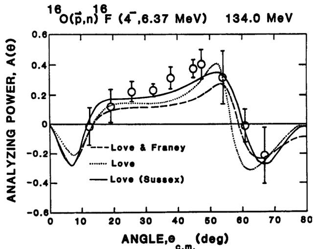
Figure 1. The angular distribution of the analyzing power for the  $^{16}\text{O}(p,n)^{16}\text{F}$  ( $4^-$ , 6.37 MeV) reaction at 134.0 MeV. The curves represent DWIA calculations with three different effective interactions as discussed in the text.
