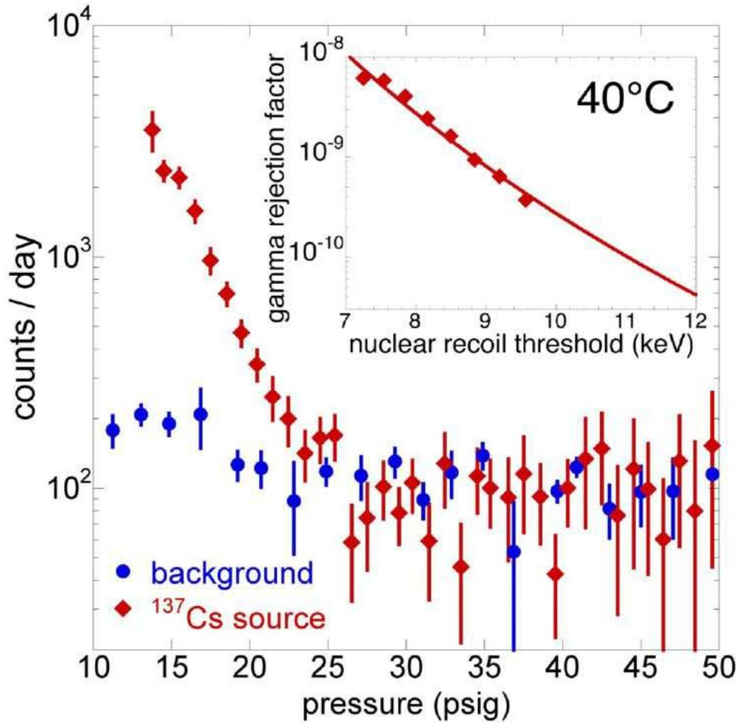
Figure 3: Response of the chamber to an intense  $^{137}\text{Cs}$  gamma source. The expected gamma interaction rate with the superheated liquid is  $3.9 \times 10^6$  per second, with gamma-induced electron energies reaching up to 662 keV. *Inset*: Intrinsic gamma rejection factor (fraction of interacting gammas inducing bubbles) obtained from the exposure to the source (see text).
