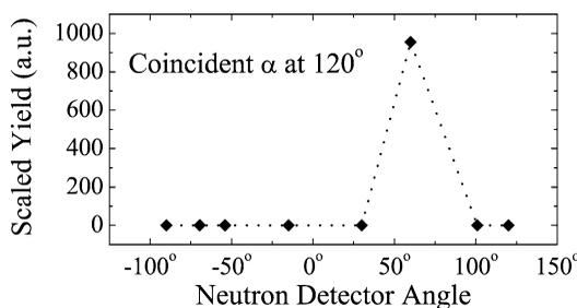
Fig. 5. The number of neutrons coincident with  $\alpha$  particles, from the Monte Carlo simulation of projectile breakup under the assumption that the entire  $\alpha$ -particle yield results from this process. The detector and experimental parameters from the one-neutron transfer simulations were also used here. The line has been placed on the graph to guide the eye.
