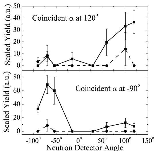
Fig. 3. The observed number of neutrons coincident with  $\alpha$  particles, displayed vs. neutron detection angle. The square points are the  $^{209}\text{Bi}$ -target data. The circular points are the mylar-backing data. Lines have been placed on the graph to guide the eye.
