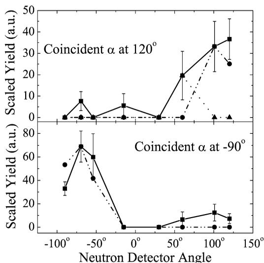
Fig. 6. A comparison of the simulated and observed coincident neutron angular distributions. The square points are the  $^{209}\text{Bi}$ -target data. The circular points are the one-neutron-transfer simulations normalized by a factor of 0.225 at 90 degrees and 0.176 at 120 degrees. The triangular points are the projectile-breakup simulation normalized by a factor of 0.02. The lines have been placed on the graph to guide the eye.
