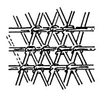
The warp is made by a pair of rods, knotted to a hoop of iron with a nylon thread. Each pair is spread at a 45° angle: The one on the right runs downwards and the left upwards. One rod goes up spirally to the hoop of iron and
