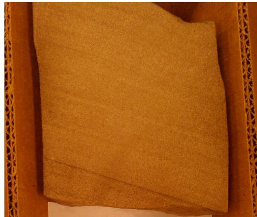
FIGURE 24. Photograph of a core from a Mumford Hills well showing the uniformity of grain size.
