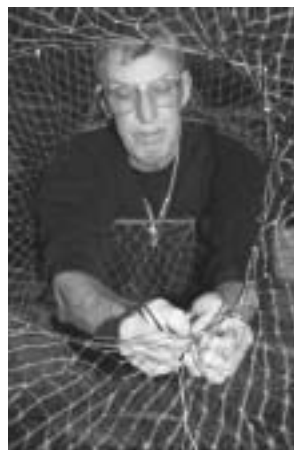
Jim knits the throat of a hoop-net from inside the net. — Photo by Rich Remsburg
