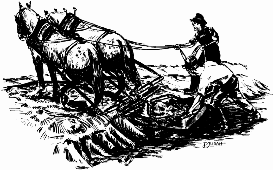
Figure 3. Horse-drawn slip scoop, one of several animal-powered forerunners of modern surface-mining machinery. From Wier, 1959, p. 11.
