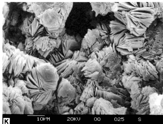
6K. Rosettes of hydrobasaluminite from above the gypsum crust on the substrate limestone. Compare with figure 5M.
