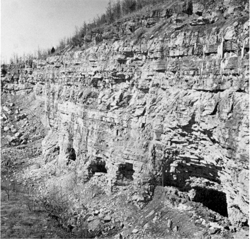
Figure 13. Abandoned underground mines near Milltown, Harrison County, where Ste. Genevieve and St. Louis limestones were mined intermittently for lime by the Louisville Cement Co. from 1903 to 1953.
