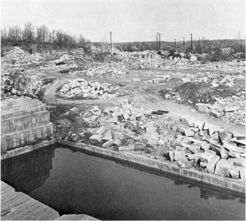
Figure 11. Waste blocks of Salem limestone at the Perry, Matthews & Buskirk (P.M. & B.) dimension stone quarry north of Oolitic. The blocks were crushed for lime burning in the early 1900's.
