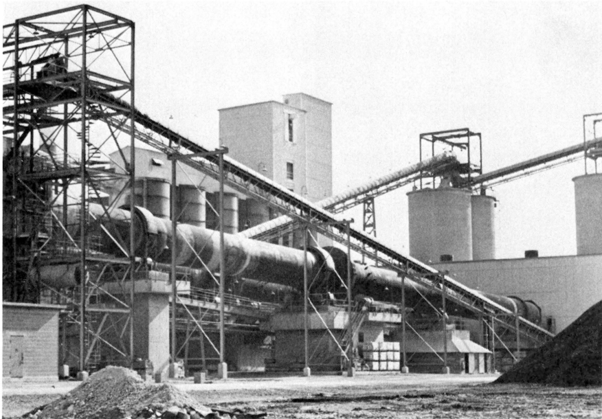
Figure 6. Modern rotary kilns at the Marblehead Lime Co. plant at Buffington near Gary.
