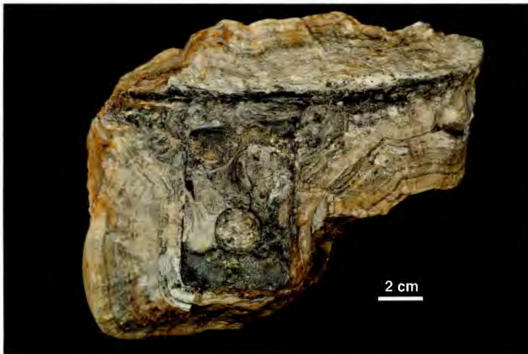
Figure 13 (cont.). Photographs of scale formed in wet limestone scrubber. C. Close-up of scale shows fibrous crystals and episodic growth of gypsum. D. Parts of the metal can adhere to scale. Minor phases contain metals.
