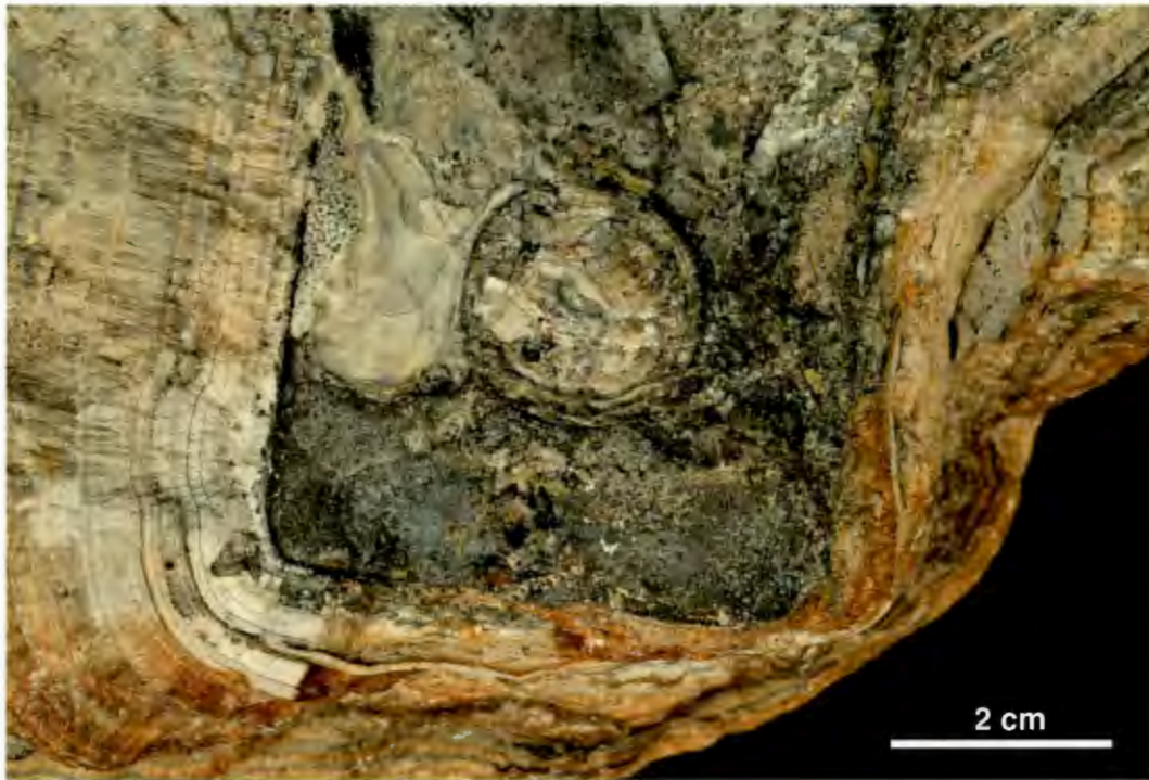
Figure 13 (cont.). Photographs of scale formed in wet limestone scrubber. E. Close-up of D showing metal within early formed scale.
